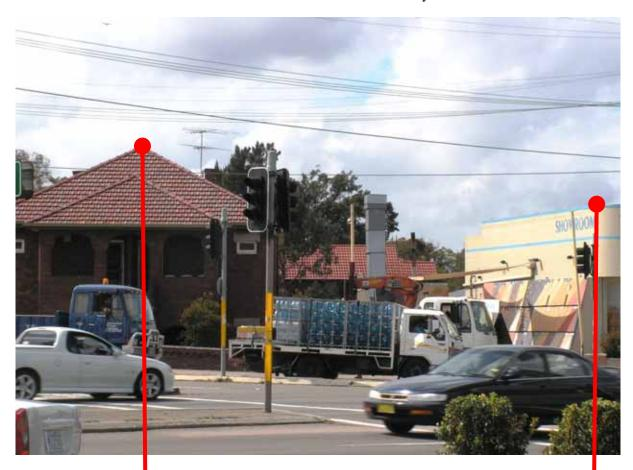
The ridge of this house is in front of the stack, and may therefore have an effect on the dispersion from the stack. It is clear that the top of the stack is probably at or just below this level—certainly not 4 m above the roof of this building which is within 50 metres.
