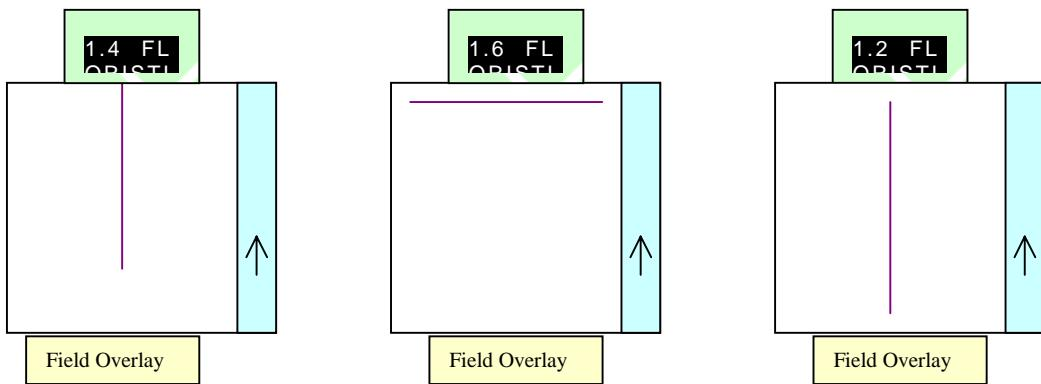
The intermediate frame will be the first photo in a run and mapping frame the second. The third frame in the run will be marked that same as intermediate frame, the forth the same as mapping frame and so on.
